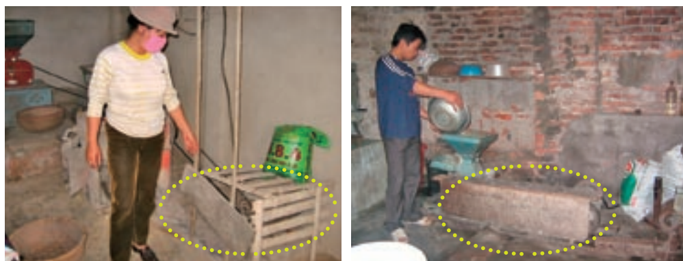
Figure 5-8. Covering moving machine belts.
