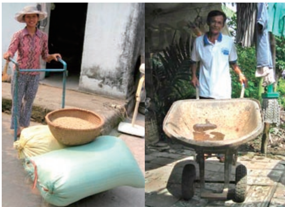
Figure 5-6. Improvement example made by farmers: Self-made hand trucks for carrying heavy materials
