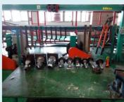
Tool racks were set up at the fitter's workstation. Tools are properly hanged and easy to reach. More space is available for operation. Abrasions between tools and molds are effectively reduced.
