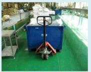
Hoppers were used to load cables instead of bags, which greatly reduced generation of wasted bags and labour costs related to unpacking and transportation (about 13,000 RMB saved annually).
