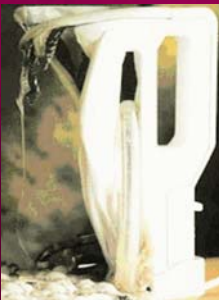
A melted, inexpensive kettle, caused by a "pirated" switch
